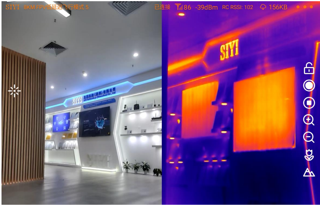
Split Image – Wide Angle Camera & Thermal Camera
